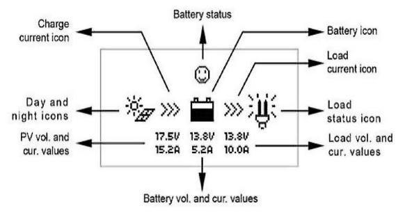
Figure: DC meter display elements
