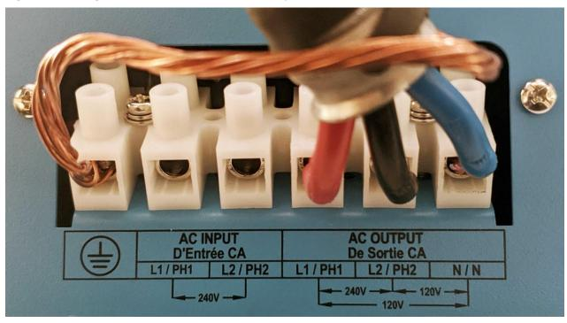
Figure: AC Wiring connections for a 2-line electrical panel
