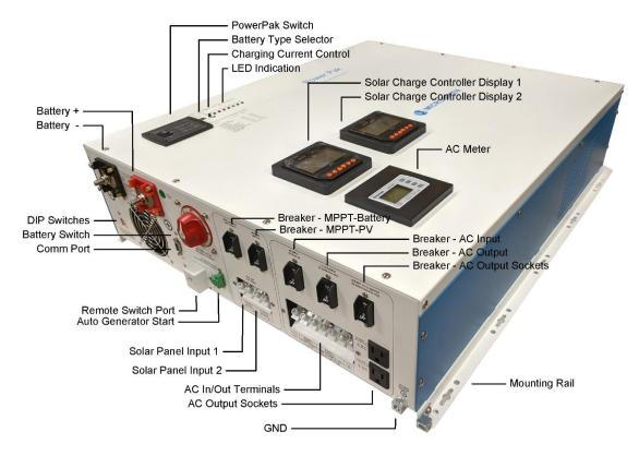
The Power Pak combines an *inverter*, *AC auto-transfer switch*, *battery charger*, and *solar charge controller* into one complete system with a peak overall conversion efficiency of 80% to 85%, with an inverter efficiency of 95%. It features power factor corrected, sophisticated multi-stage charging and pure sine wave output with unprecedented high surge capability to meet the demanding power needs of inductive loads without damaging the equipment.
