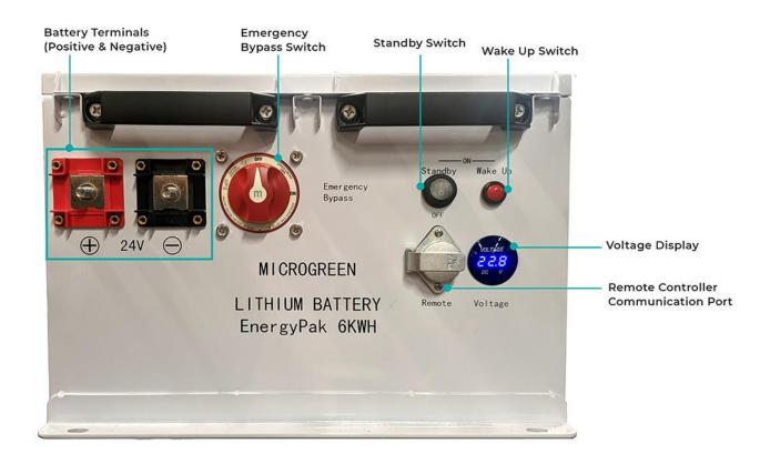
Figure 3a: Front panel components of the 6 kWh Energy Pak (Note: same elements available on the 3 kWh Energy Pak)
