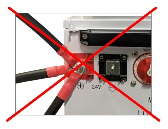
Figure 5b: Incorrect connection for multiple loads (multiple wires directly connected to the battery terminal)
